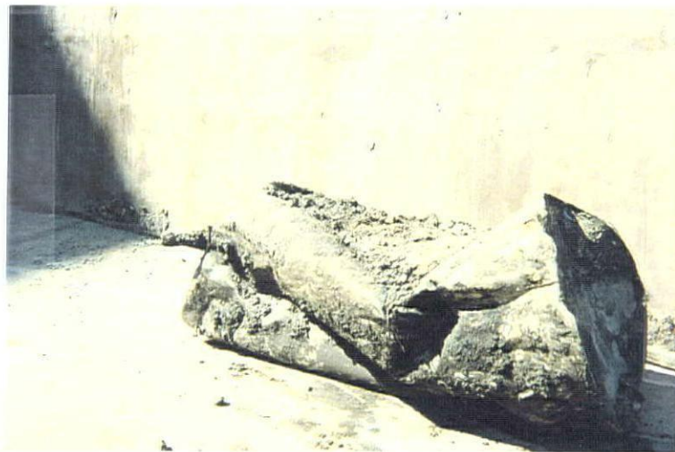
Figure 4: Pictures of the First UST (550 Gallons) removed from the Virginia Power (City Hall Avenue) Substation in Norfolk, Virginia.
